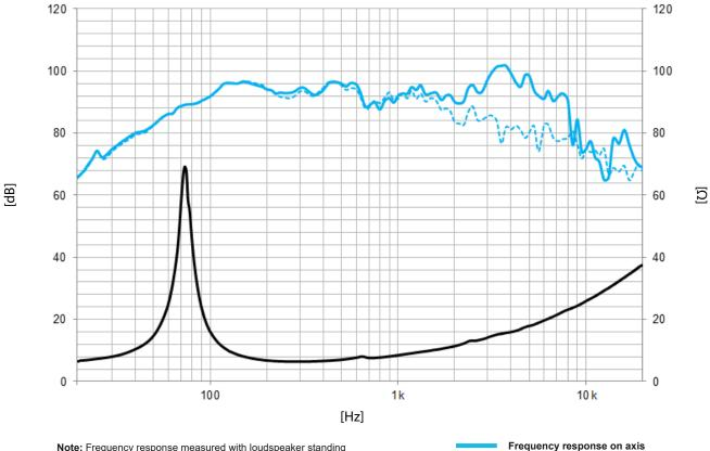
Note: Frequency response measured with loudspeaker standing on infinite baffle in anechoic chamber, 1W @ 1m  $\,$
