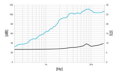
Note: On axis frequency response measured at 1W /1m
